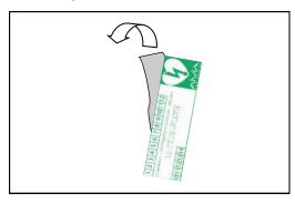
$\bullet$  Stick the seal covering both the AIVIA door and chassis
