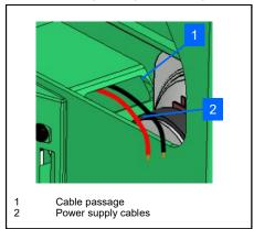
• Connect cables to the supply terminals, respecting proper polarity.
