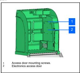
• Unscrew the fixing screw with a phillips screwdriver and pull out the hatch from the top.
