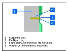
Washer plus screw head thickness must not exceed 8mm.(0,31 in)
