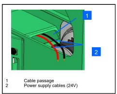
• Connect the cables on the connector block respecting the polarity.
