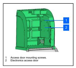
Unscrew the fixing screw with a Philips screwdriver and pull out the hatch from the top
