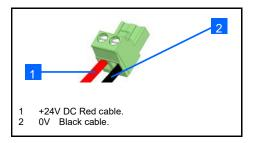
• Plug the connector block onto the board.
