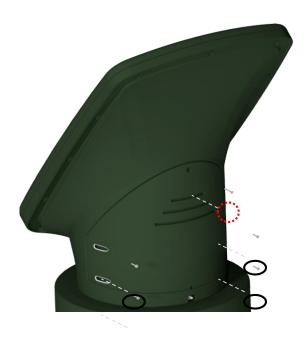
Reattach the rear hatch using the screws provided. Caution: one of the screws (marked here in RED) is  $5 \times 30$ , i.e. longer than the other 4 screws, which are  $5 \times 20$ .
