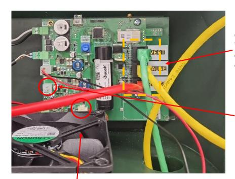
Connect the GREEN, RED, and YELLOW RJ45 cables to the circuit board according to the colours printed on the board.
