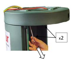
Before connecting and positioning the head on the cabinet, detach the rear hatch by removing the  $\mathbf{5} \times \mathbf{30}$  Phillips screw:
